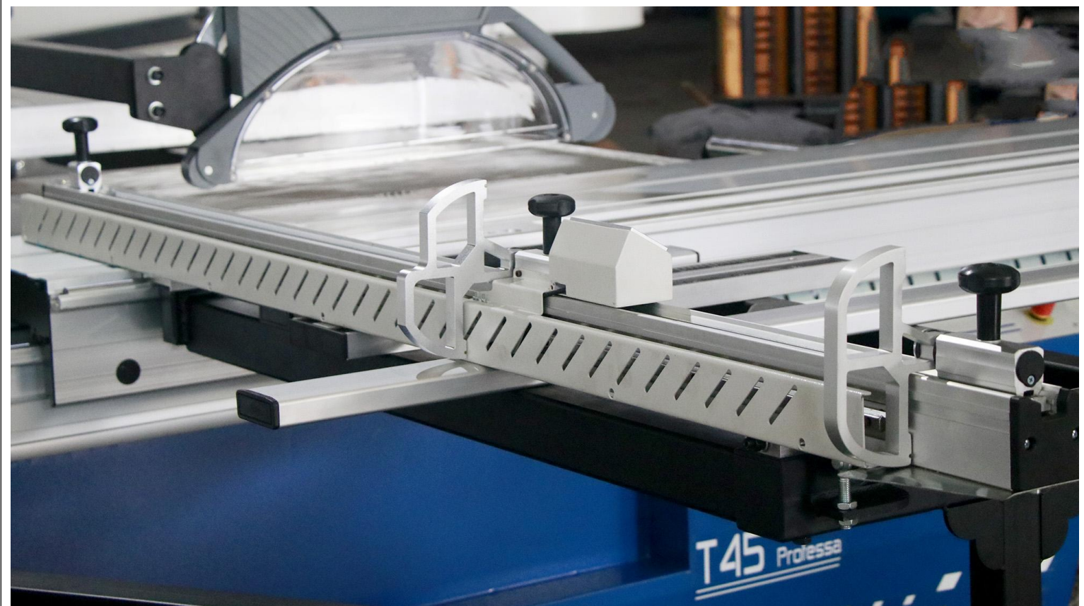
ENG T45 cross cutting ruler is a digital display model, with linear guiding rail to guide the sliding of stop, max measurements up to 3660mm
