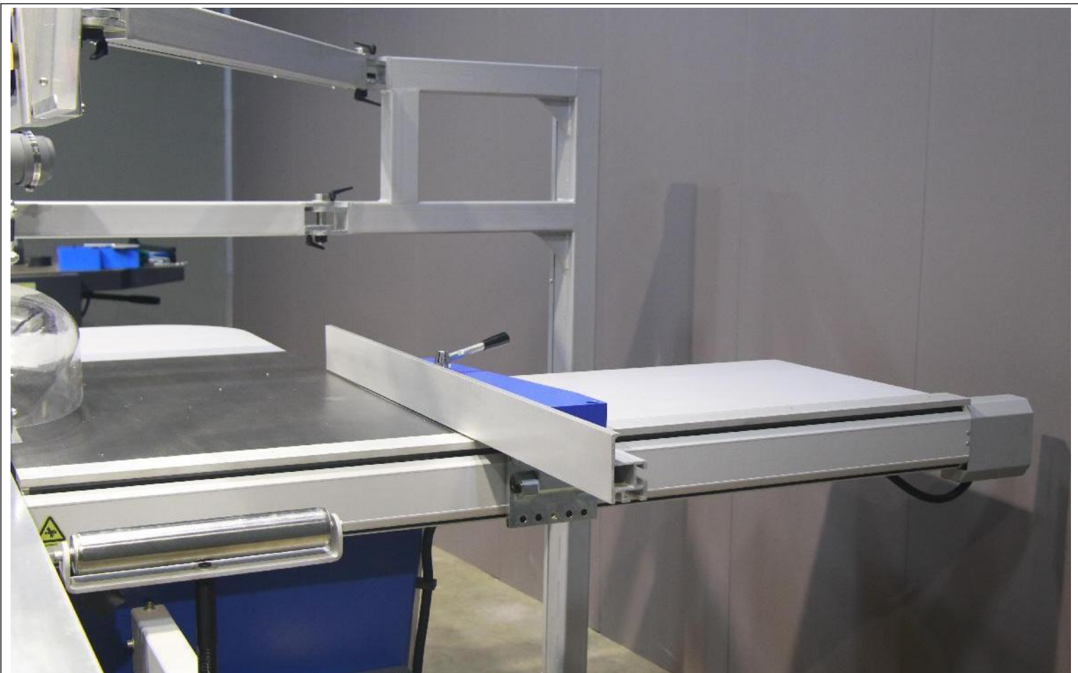
Max 1300mm rip cutting capacity the rip cutting fence is absolute servo drive, highest precision for repeat positioning.
