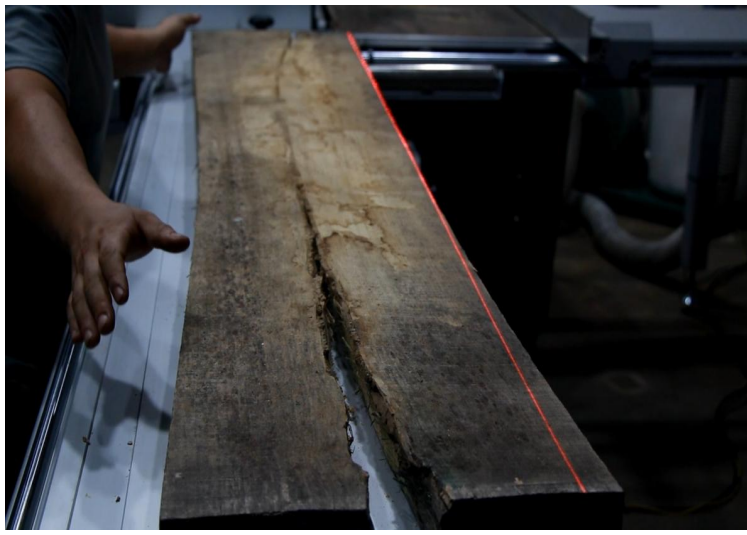
Optional laser line for easy reference of rip cutting, also notice the user where the blade is, makes cutting safe
