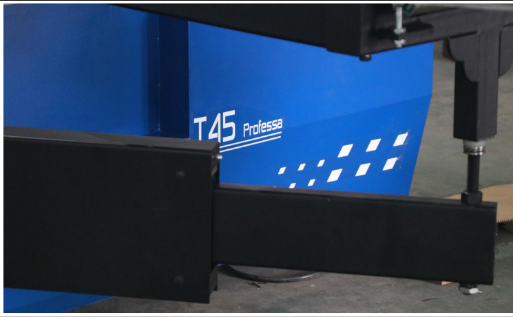
To avoid bending at extreme length, the supportive arms we applied steel rather than aluminum, after straighten and grinding on surface
